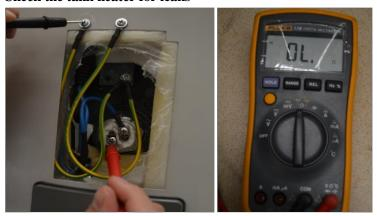
Press the yellow button to switch to the picture shown, turn the heating power measurements, if leakage resistance is zero, if not leak, show resistance.
