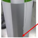
After the Cover is removed, use a screwdriver to remove the bottom two screws of the Front cover – down.
