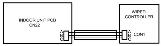
Note:When do the wired controller & indoor PCB wiring work for model ADH071M3ERG,do not connect the shielded wired to the unit's shell,do not parallel wiring with strong electric lines within 0.3 meters, please keep strong lines and the signal lines separately.
