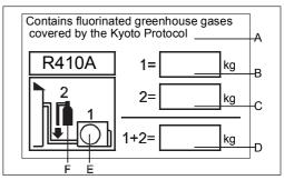
This product contains fluorinated greenhouse gases covered by the Kyoto Protocol.Do not vent into the atmosphere. Refrigerant type:R410A
