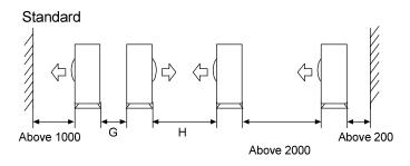
The top and two side surfaces must be exposed to open space, and barriers on at least one side of the front and back shall be lower than the outdoor unit.
