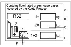
This product contains fluorinated greenhouse gases covered by the Kyoto Protocol.Do not vent into the atmosphere. Refrigerant type:R32
