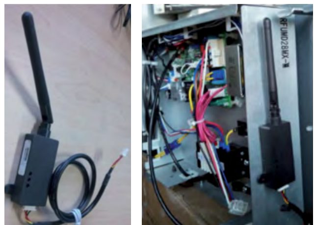
Radio adapter for the indoor unit to be connected to the respective electronic board.
